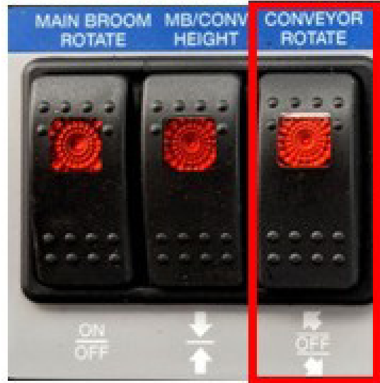
Fig. 64: Conveyor Rotate Switch
