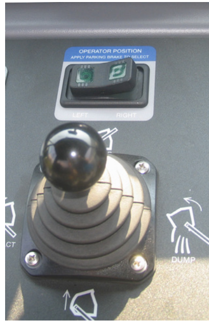
Fig. 125: Operator Position Switch
